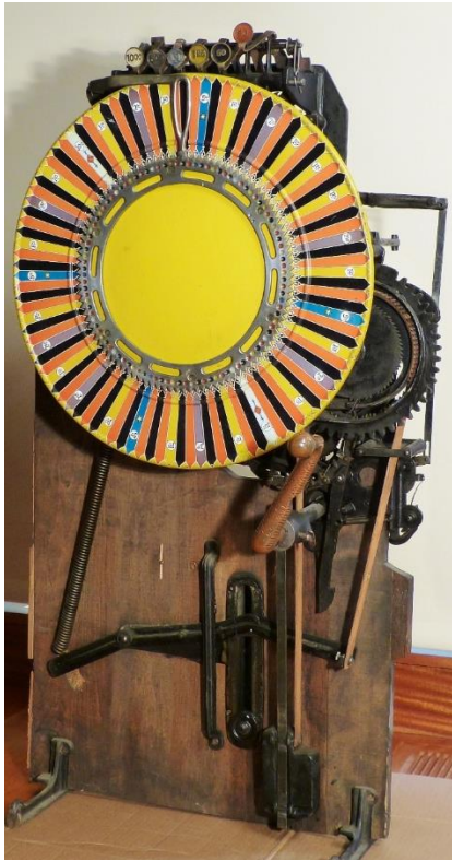
Mechanism Photos of Gabel's Chicago Upright Slot Machine: front, back, left side, right side. This is very different than the mech from any other manufacturer. Rick Crandall collection.
